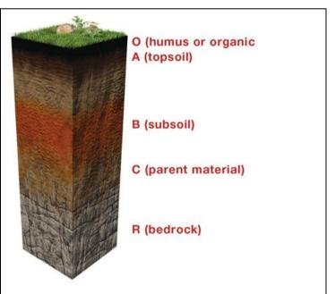
**Figure 1.** Soil profile, distributed in layers or horizons (A, B, C and R). Most soils have three major horizons (A, B, C) and some have an organic horizon (O) also called humus. Source: Soil Science Society of America, 2015
